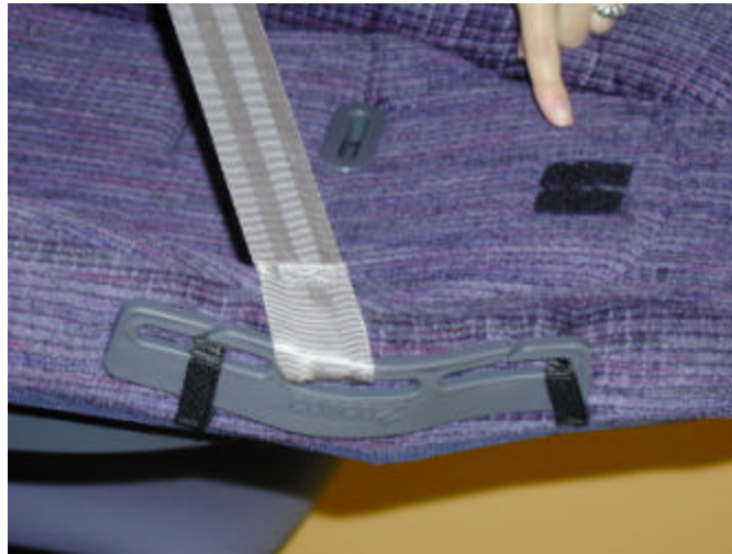
Webbing looped at comfort guide; Velcro on back of seat to hold Alex's head
